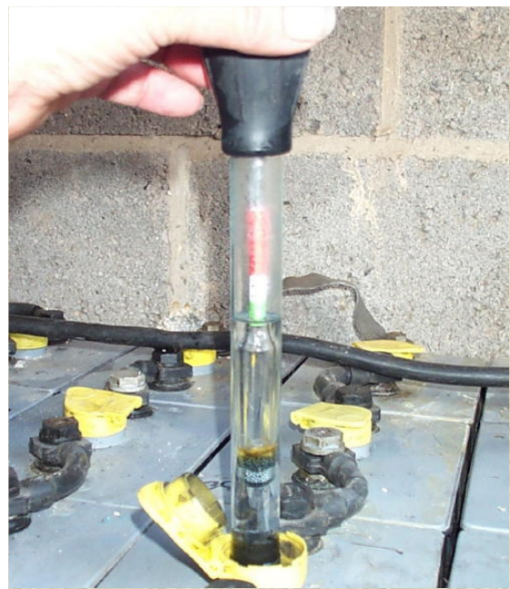
testing the specific gravity of the electrolyte in a cell with a hydrometer
