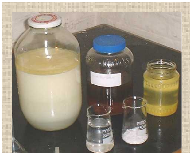
ingredients and by-products: clockwise from left – wash-water, glycerine, finished biodiesel, potassium hydroxide, methanol
