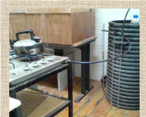
using biogas to boil a kettle on a normal hob - the only difference is there's no gas bill.
