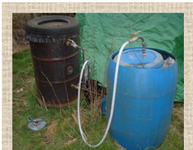
small experimental biogas digester at Redfield. Waste material is put into the oil drum, neoprene cover rises when full of gas, gas is tapped into container (upside-down plastic drum with water seal) which rises as more gas enters. When full, gas can be tapped off and used with the little gas ring.
