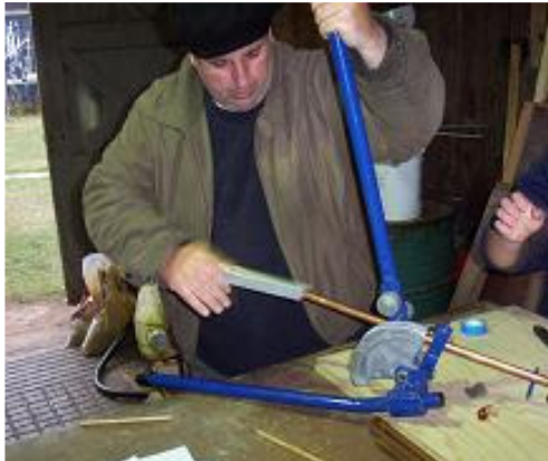
getting to grips with a pipe bender; books are sometimes not enough - you have to have a go
