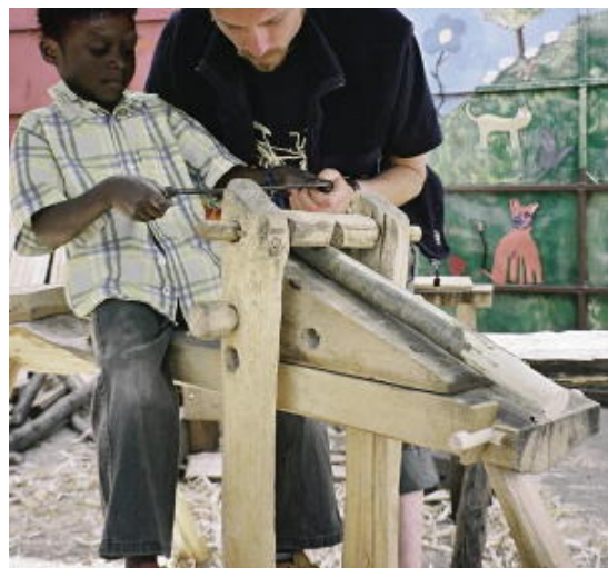
using a shave horse and draw-knife to roughly shape a chair leg; the techniques required are easily learned by all ages and skill levels.
