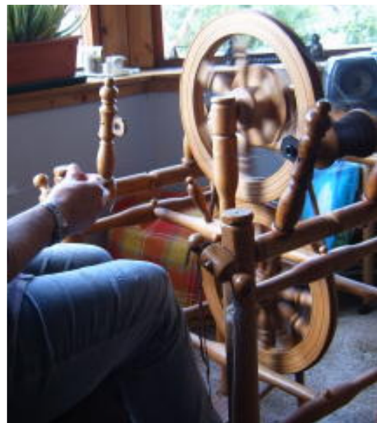
'chair' wheels were originally made from old chairs turned upside down; made of oak and held together with pegs, this one has 2 wheels linked with a belt, to save space.
