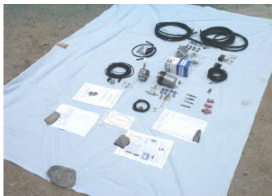
all the kit required for an Elsbett conversion of a Citroen ZX.
