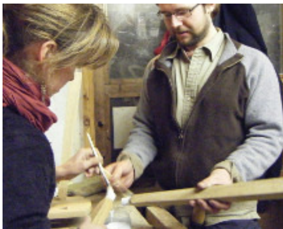
applying PVA glue to a round-tenoned stool leg
