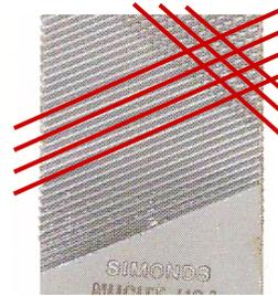
**Double-Cut** files have two sets of diagonal rows. The first set is called the overcut. The second set is cut at a different angle with the file axis, and is known as the upcut (it is finer than the overcut).
