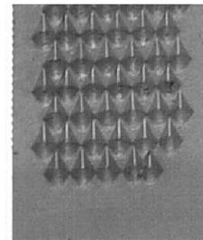
**Rasp-Cut** is a pattern where each tooth is individually formed by a single-point tool or punch - the teeth are formed separately and are disconnected.
