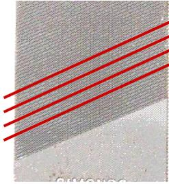
**Single-Cut** files have a single set of diagonal rows of teeth, parallel to one another and extending across the working face of the file.
