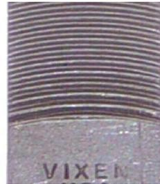
**Curved-Cut** is an arrangement of file teeth in curved contours across the working face of the file. The teeth are milled with a decided undercut (or positive rake).
