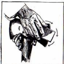
Fig. 12.—Hone with a circular motion of the stone.
