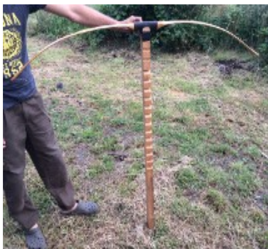
Using a tillering stick to check the symmetry of the bend in the bow.
