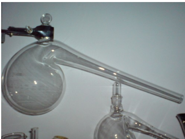
A retort – old-style 'alchemical' distillation equipment, superseded since the invention of ground glass joints; the new equipment is easier to use and clean, and increases yields.
