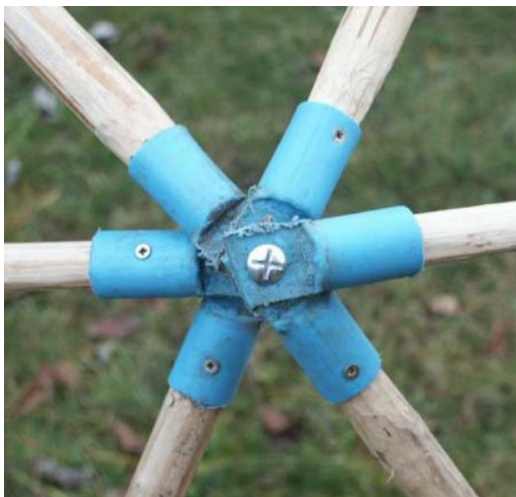
One method of connecting poles for a home-made geodesic tent frame.
