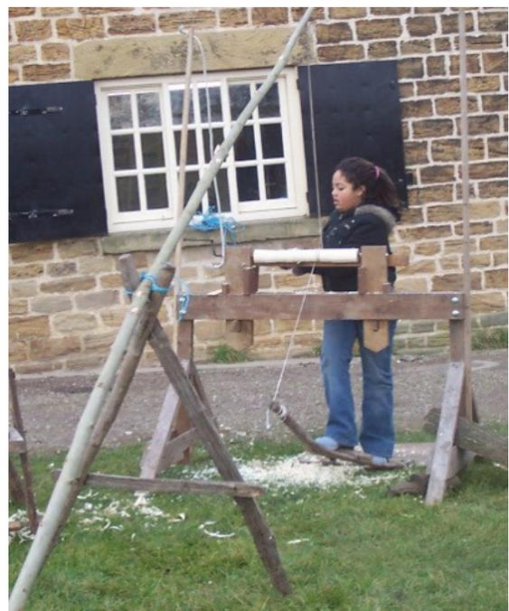
*Using a pole lathe.*
