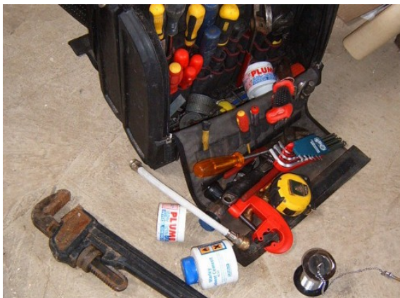
A basic plumbing toolkit, including a stillson wrench, pipe cutter, solder and flux (used to help the solder spread into the joint).
