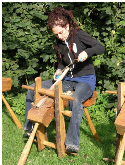
Using a shave horse and draw knife to cut a peg roughly to size.
