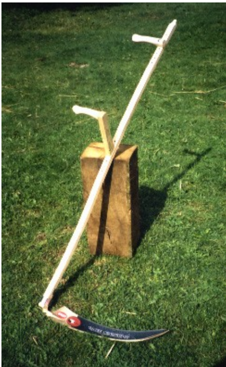
An adjustable wooden snath, with a 60cm Austrian-style blade.
