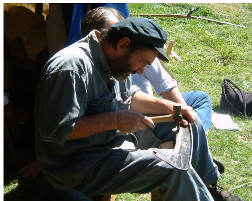
Peening – cold forging the blade to make it thinner and sharper.
