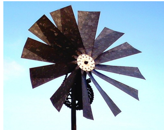
Small home-made windmill for pumping water.
