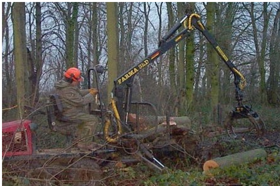
Lightweight, 8-wheel drive 'forwarder' – it forwards timber from the felling site out to the stack; this can also be done by horses.
