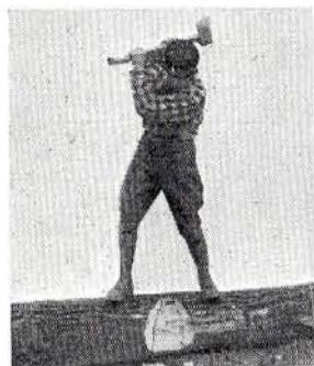
Fig. 19.—Position of hands and axe at Top of Stroke. Note that the head is down—eyes on the cut.
